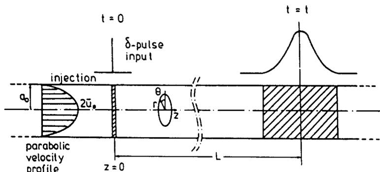
Fig. 1. Schematic diagram of the dispersion profile of the sample through the chromatographic tube, in the ideal Taylor dispersion experiment. From Ref. 11.
